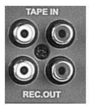
The TAPE IN sockets allow cassette recorders or CD players to be added to the Main output. The RECORD OUTPUT provides a signal output to a cassette deck and home audio equipment. Sockets are RCA Phono.
